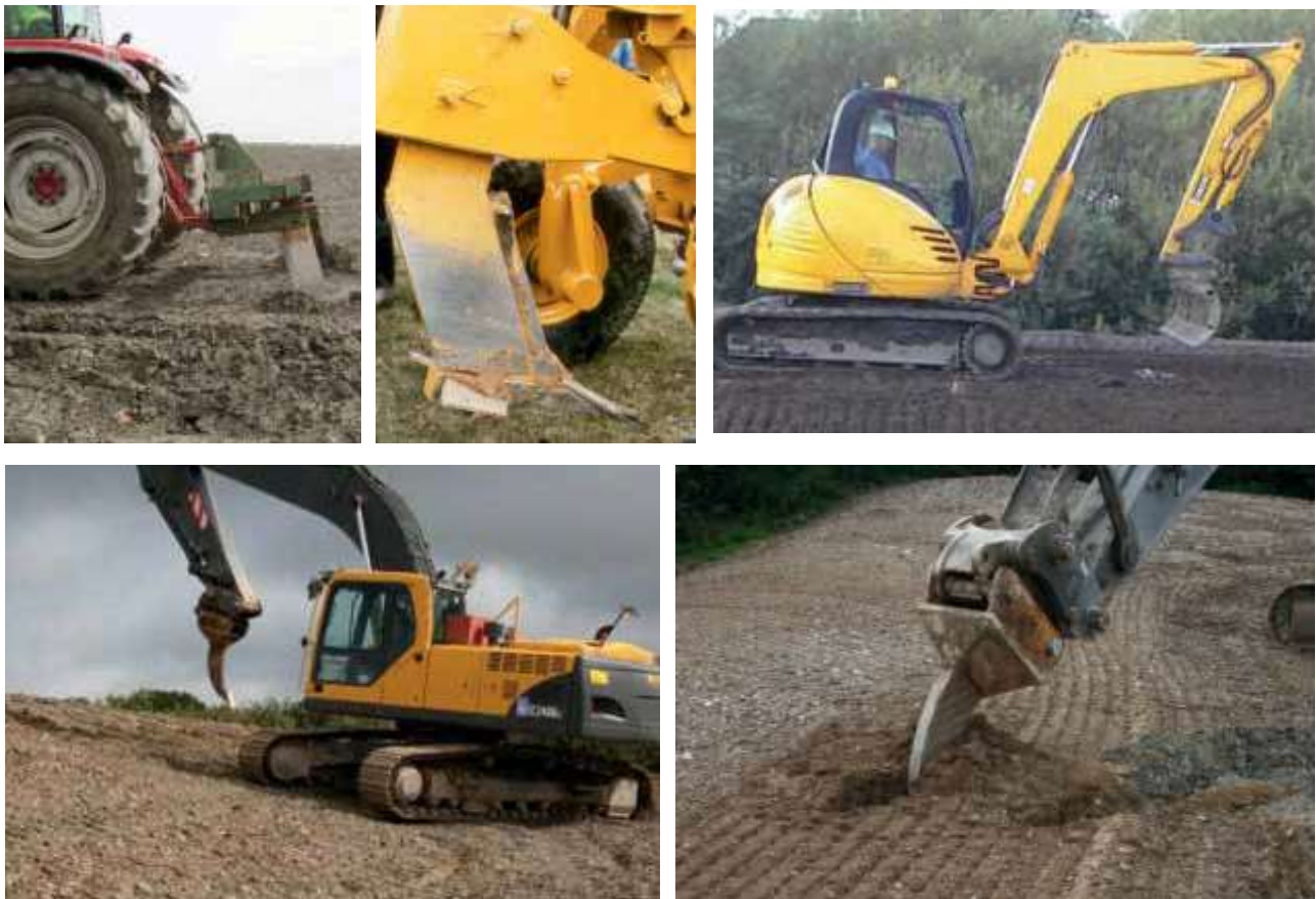
Top (from left to right): Ripping by tractor-drawn tines, Large winged-tine ripper, Topsoil rake used on a 3 tonne excavator
