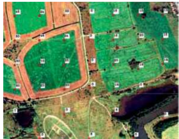
Topsoil map of a proposed development site, showing variation in thickness (cm).
